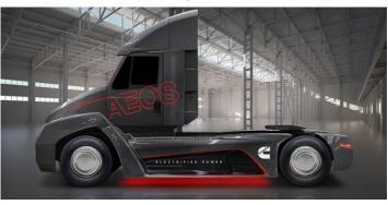
The Cummins Class 7 electric truck prototype is dubbed AEOS - one of the horses that pulled the golden chariot of Helios across the heavens every day in Greek mythology. It has a 145 kWh battery and can haul a 22 ton trailer for up to 100 miles. Thanks to its advanced technology, recharging takes only an hour using a 140 kW charger. **{more}**
